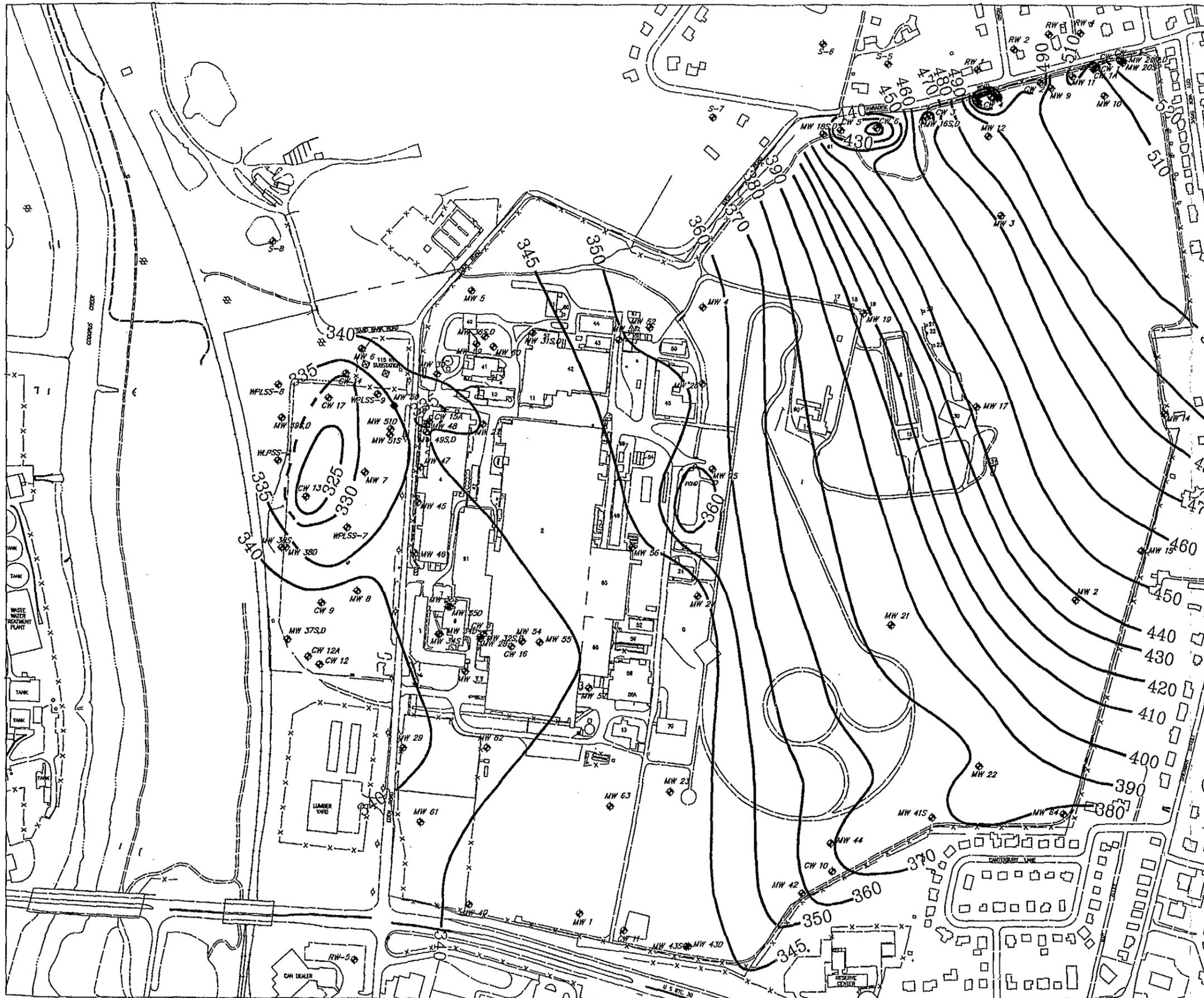
11/6/97 GROUNDWATER SURFACE ELEVATIONS & APPROXIMATE DAILY PUMPING RATES FROM "CW" WELLS
